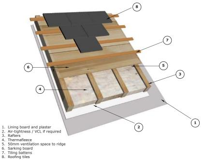
Tiling battens Roofing tiles
